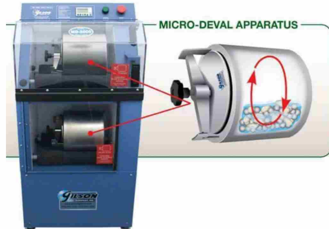
Figure 2. Picture of the Micro-Deval Test Apparatus illustrating the concept of the test 7 .
