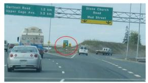
Figure 19 - Freeway Exit sign Partially Eclipsed by the Object Marker Warning Sign (View South from the Mainline)
