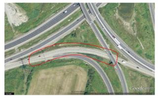
Figure 26 - Outside Lane Ends within Horizontal Curve
