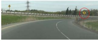
Figure 30 – Inappropriate Merge Warning Sign (View North from On-Ramp)
