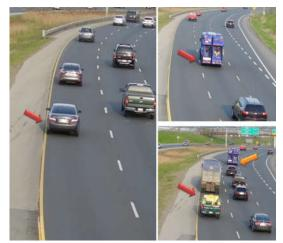
Figure 16 - Observed Cases of Swerve- and Overcorrection-Manoeuvers (View West from Pritchard Road Overpass)
