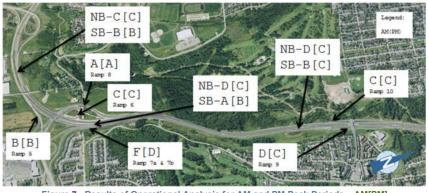
Figure 7,- Results of Operational Analysis for AM and PM Peak Periods - AM[PM]
