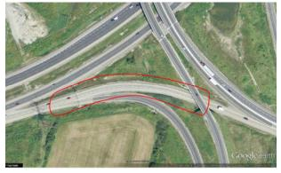
Figure 24,- Outside Lane Ends within Horizontal Curve
