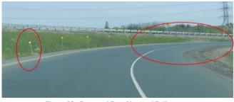
Figure 30, - Damaged Post-Mounted Delineators
