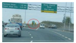
Figure <u>15,- Freeway Exit sign Partially Eclipsed by the Object Marker Warning Sign (View South from the</u> Mainline)
