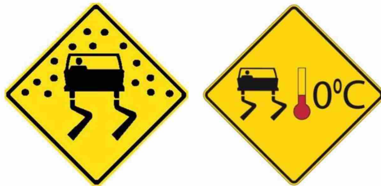
Figure 23: SLIPPERY WHEN WET sign (left) and BRIDGE/ROAD ICES sign (right)
