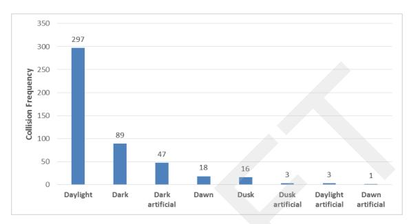
Figure 3: Collisions by light condition
