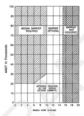
Figure 29: Median Barrier Warrant Guide for Divided Highways
