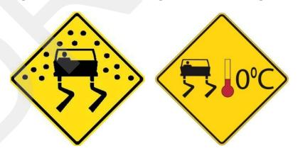
Figure 23: SLIPPERY WHEN WET sign (left) and BRISGE/ROAD ICES sign (right)
